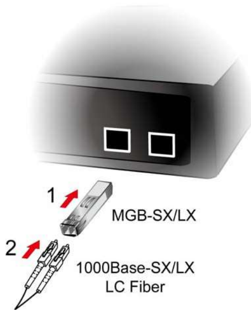
Figure 2-1-7 Plug in the SFP transceiver
