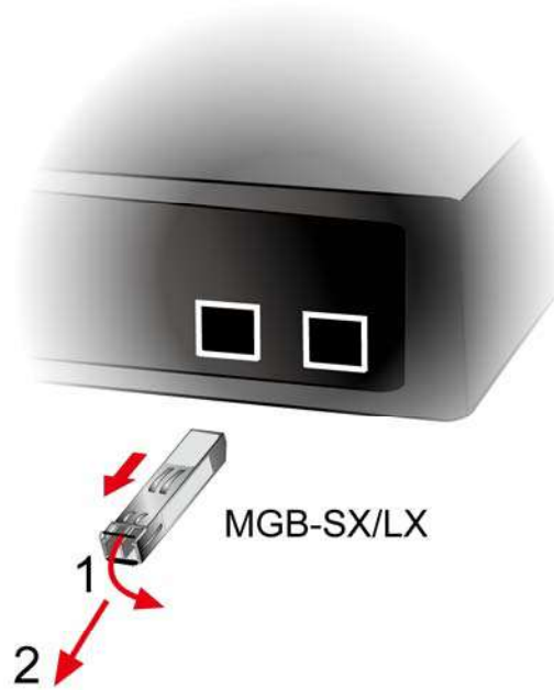
Figure 2-1-8 How to Pull Out the SFP Transceiver
